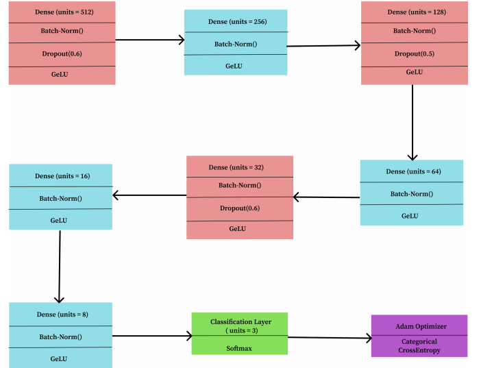
Fig. 4. Architecture of Multi-layer Artificial Neural Network (ML-ANN)
